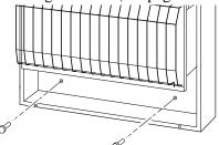
Figure 12 - Installing Bottom Mounting Screws
